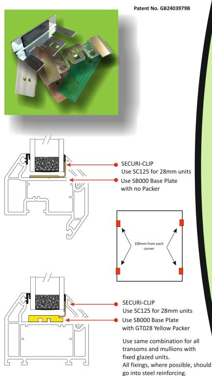
All drawings are not to scale Reinforcement and fixings have been omitted for clarity UK Fasteners screws were used for testing when required **GT SECURI-CLIP** is a patented glass retention system which, when fitted in the appropriate numbers and position, assists internally and externally beaded windows and doors to meet the requirements of PAS 23/24.
